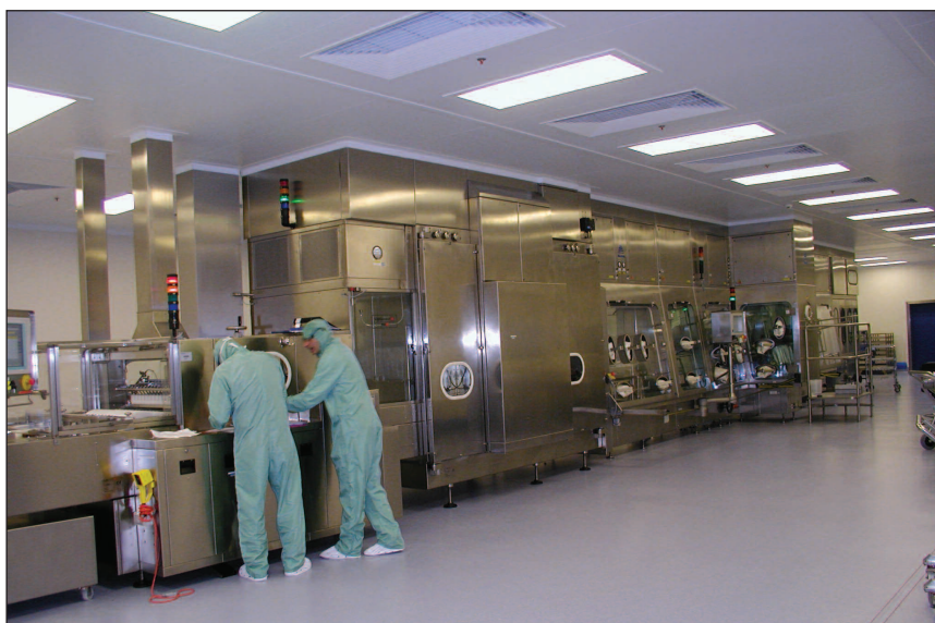
Figure 1 – A complete aseptic vial filling line using a unidirectional air flow isolator for the filling process, and a RABS for the capping stage
