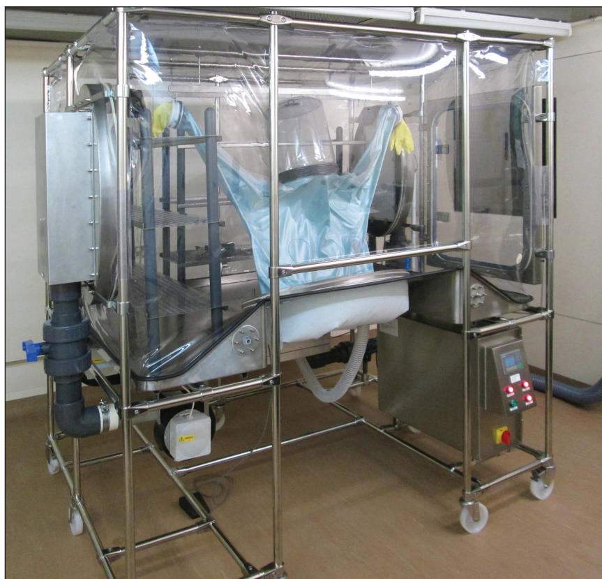
Figure 3 – A flexible film half-suit isolator for sterility testing, specially-designed for use in a room with a low ceiling, the HEPA filters therefore being mounted on the walls of the canopy. The control system maintains a set canopy pressure via two-fan ventilation, and provides digital display and alarms on the air flow rate and the canopy pressure.
