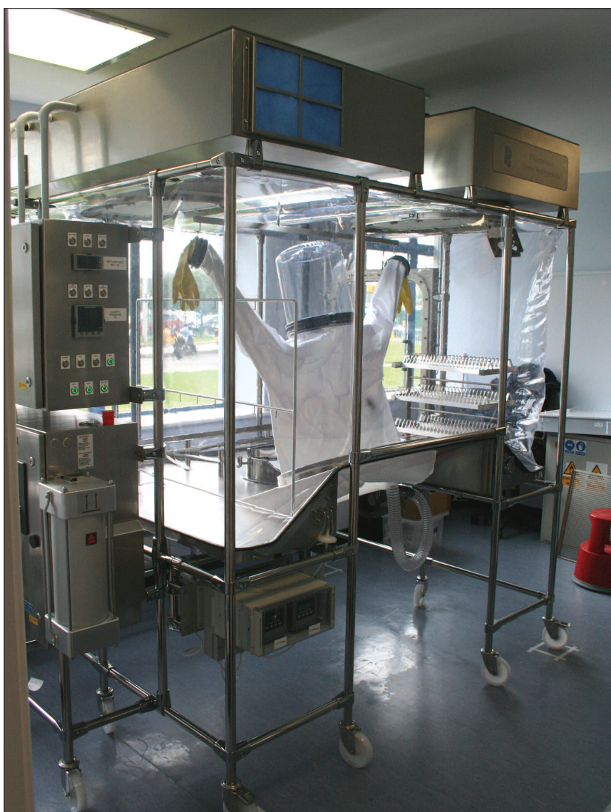
Figure 2 – A flexible film half-suit isolator designed for sterility testing, using roof-mounted HEPA filters for turbulent air flow, and fitted with an on-board hydrogen peroxide vapour generator for bio-decontamination. This isolator also incorporates instrumentation of the hydrogen peroxide concentration at both high and low levels.
